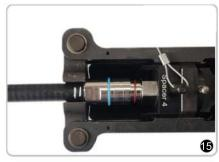
Make sure the connector nut is lined up against spacer 4 to prevent damage to the O-ring during compression.
