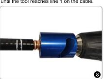
Using the low speed setting on the drill, insert exposed outer conductor into trimming tool base. Continue trimming until tool reachescable jacket. Do not push tool beyond this point.
