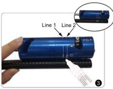
Align the end of cable with the end of trimming tool and make two marks on the cable jacket that correspond with lines 1 and 2 on the trimming tool.
