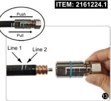
Push the connector onto the cable past Line 2. Then pull the connector to make sure the connector cannot be removed. It will stop just right of Line 2 automatically.
