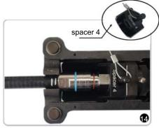
Place spacer 4 into the compression frame. Make sure the connector and cable both lay flat in the compression frame. Make sure the flat side of connector is upwards.
