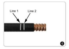
Use the "flat end" of foam remover for outer conductor and dielectric preparation. Rotate back and forth to prepare outer conductor and compact the foam dielectric.
