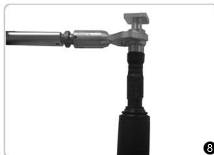
Tighten with torque wrench. Recommended torque is 5N·m.
