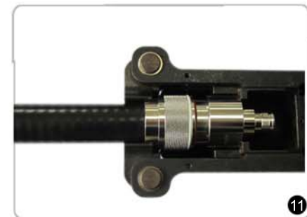
Put the connector into the compressing frame and make sure connector being sitted steadily.
