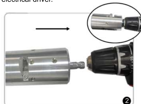
Attach the trimming tool to power drill.
