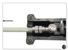
Make sure the connector nut is lined up against spacer 3 to prevent damage to the O-ring during compression.
