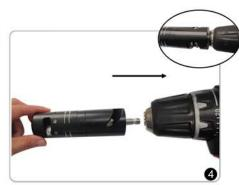
Assemble the trimming tool to power drill.
