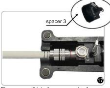
Place spacer 3 into the compression frame. Make sure the connector and cable both lay flat in the compression frame.
