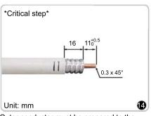
Outer conductor must be prepared to the crest in the corrugation as shown.
