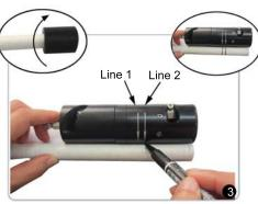
Assemble the cap. Align the end of cable with the end of trimming tool and make two marks on the cable jacket that correspond with lines 1 and 2 on the trimming tool.
