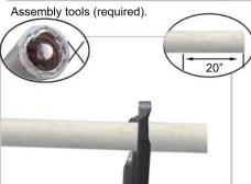
Straighten the first 20 inches of the cable, and proceed to cut the cable with cable cutter at the valley (low point) of the corrugation.
