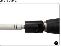
To create the chamfer shown in critical step, push the power drill with back part of trimming tool at low speed or 400 RPM until the leading surface of trimming tool reaches the cable jacket.
