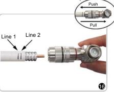
Push the connector onto the cable past Line 2. Then pull the connector to make sure the connector cannot be removed. It will stop just right of Line 2 automatically.
