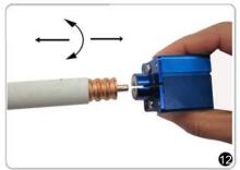
Use the foam remover to rotate it in CW/CCW alternately and pull to remove any dielectric residue.
