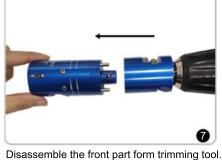
assemble to the power drill.
