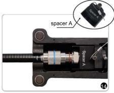
Place spacer A into the compression frame. Make sure the connector and cable both lay flat in the compression frame. Make sure the flat side of connector is upwards.
