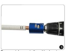
To prevent damage to the cable, do not push the trimming tool beyond the end of the cable jacket.
