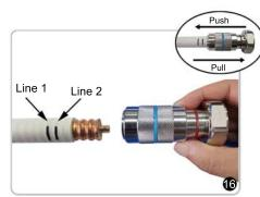
Push the connector onto the cable past Line 2. Then pull the connector to make sure the connector cannot be removed. It will stop just right of Line 2 automatically.
