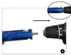
Attach the trimming tool to power drill.
