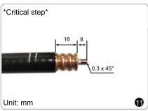
Outer conductor must be prepared to the crest in the corrugation as shown.
