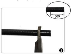
Straighten the first 500mm of the cable, and proceed to cut the cable with cable cutter at the valley (low point) of the corrugation.
