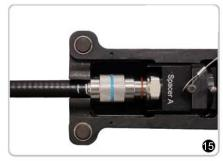
Make sure the connector nut is lined up against spacer A to prevent damage to the O-ring during compression.
