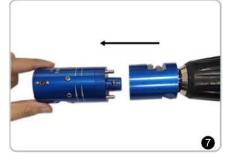
Remove the front part of trimming tool from the base. The base will remain attached to
