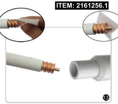
Hold cable end at a downward angle,tapping the cable while vacuuming.Clean the inner and outer conductor with alcohol pad.
