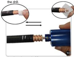
Use the other end of foam remover to remove any dielectric residue from the inner conductor. Clean the inner and outerconductor with alcohol pad
