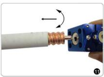
Attach the foam remover to the cable. Rotate it in CW/CCW alternately to remove the burrs of the outer conductor.
