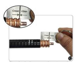
Place the depth gauge on the outer conductor. The crest of the final corrugation should be **within** the area indicated by the depth gauge.
