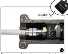
Place spacer A into the compression frame. Make sure the connector and cable both lay flat in the compression frame. Make sure the flat side of connector is upwards.
